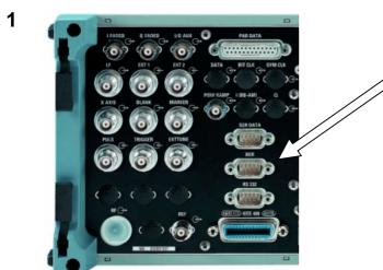
Connect the SUB-D connector of the BERT cable (1110.3551.00, delivered with SMIQB21) to the BER socket on the rear side of the SMIQ
